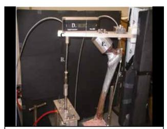
**The Dynamic Model** Figure: A. Pneumatic Pressure Cylinder B. Body Weight Force C. Aluminium Plate for visual indication of pelvis D. Digital protractor E. Artificial Acetabulum F. Iliotibial band/ abductor muscles (3/16" steelcable).
